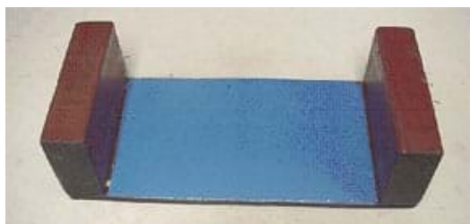
Figure 5. Wooden support structure for the testing station. Blue represents the water below the bridge. The end blocks represent bridge abutments.
